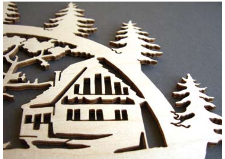
Extremely fine contours due to contactless cutting
