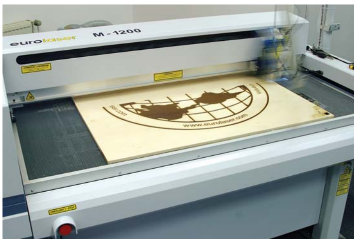
Raster engraving in wood on eurolaser M-1200
