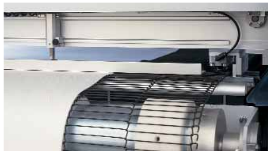
Materials handling with automatic pneumatics for material and conveyor adjustment
